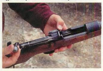
Several other features changed during the evolution from the pre-'98s to later '98s. The '98 cocks on opening, and the pre-'98s cocked on closing. The '98s have an added "safety" lug on the bolt; the pre-'98s lacked this feature.
